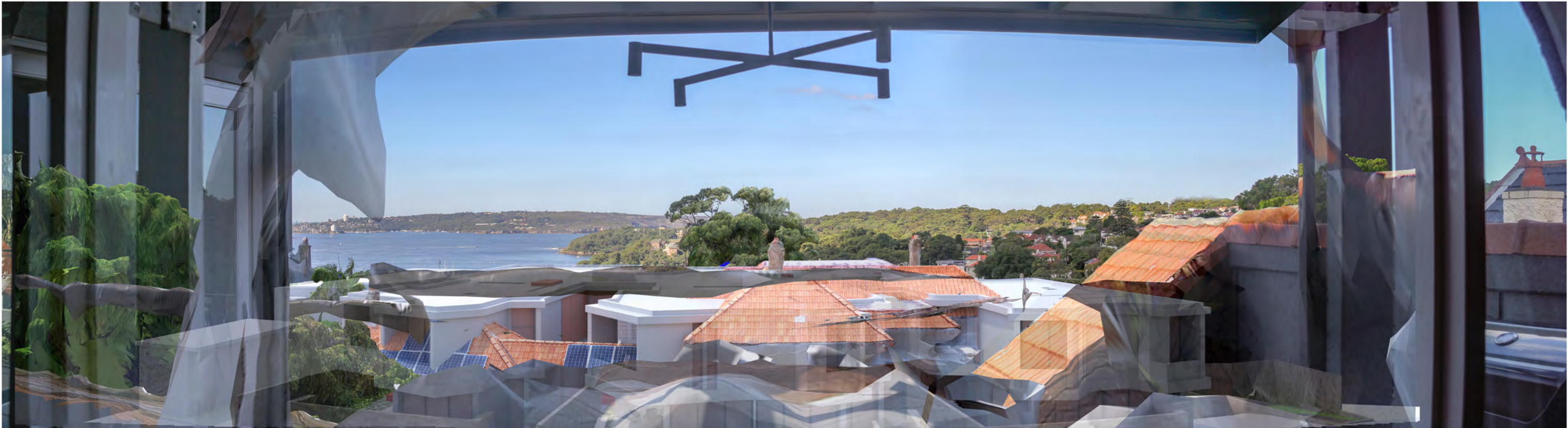
viewpoint 55 - photogrammetric drone survey information overlaid onto background photo with CAD model of new proposal positioned within the 3D survey
