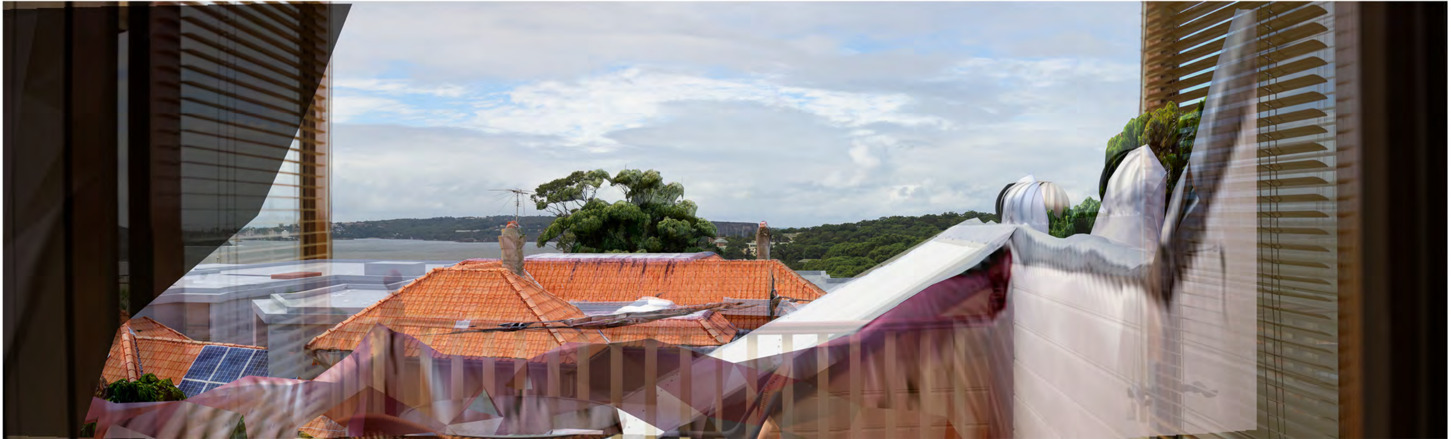
viewpoint 30 - photogrammetric drone survey information overlaid onto background photo with CAD model of new proposal positioned within the 3D survey
