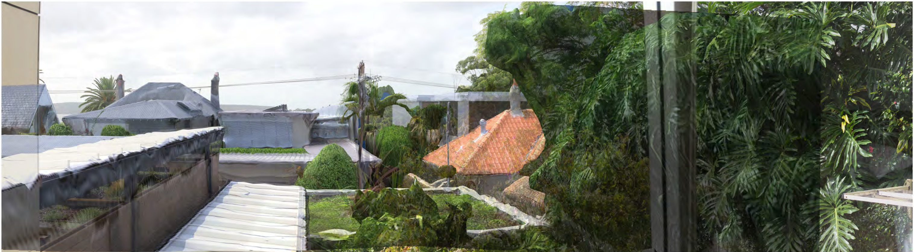
viewpoint 29 - photogrammetric drone survey information overlaid onto background photo with CAD model of new proposal positioned within the 3D survey
